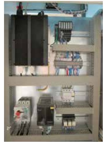
CNC OPENcontrol with I/O OPENrio SL modules.
