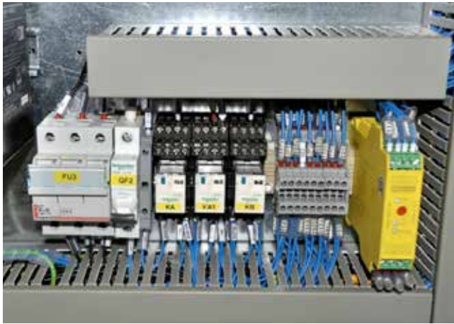
Optional module for the safe management of the machine emergencies.
